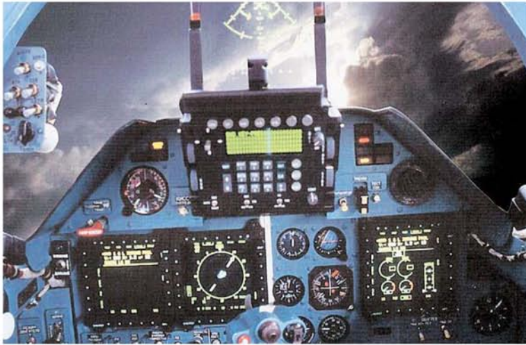
The cockpit of the Sukhoi-30 fighter, showing the pilot's Multi-Function Displays. These will now be replaced by Samtel displays, manufactured in Ghaziabad
